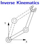
**Given**: Desired position and orientation of end-effector, **p**. **Required**: Joint Variables **q** ( $\theta$  or d) to get **p**
