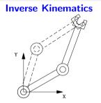
**Given**: Desired position and orientation of end-effector, **p**.
